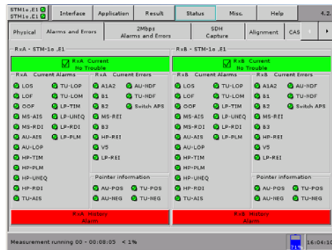
Fig.3: The CMA 3000 gives you a quick overview of errors and alarms of both sides of the SDH line.
