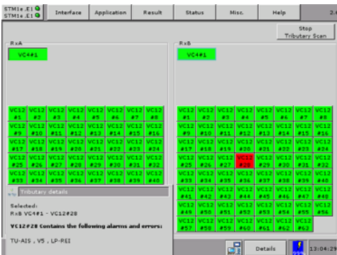
Fig.4: The trouble scan feature gives you a quick overview of the tributaries of the monitored line.
