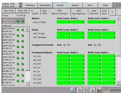
Fig. 4 The CMA 3000's color indications make it easy to identify alarms or errors in the monitored signal
