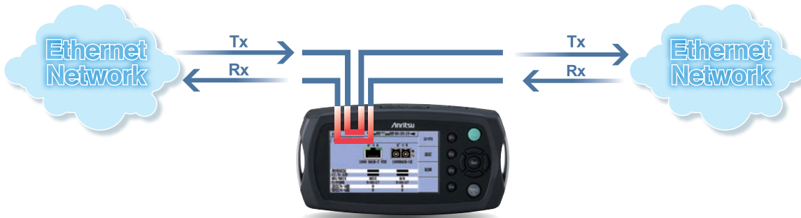
Pass through monitoring by inserting the tester in a network. Tx and Rx of two ports are used for this application.
