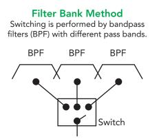
The filter bank technique uses a set of Band Pass Filters (BPF), and these each have typically a bandwidth of 400 MHz. A switch is then used to select a matrix of different BPF to give the required high band selectivity. These filters are implemented using printed circuit techniques, to give low cost, low power consumption, and high stability. The stability comes from there being no tuneable or variable circuits involved.
